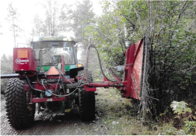
Denny Manner used the brush hog several days covering only a couple miles a day. Part of the slowness is due to bumpy trail, which makes the cutter bounce and cut unevenly.
