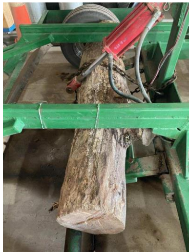
The drag broke out on the trail with Mike driving. Greg called Dan White, who was out with the Dubie sickle. Fortunately some hunters came by and helped cut a log to put between the axle. Dan used the bucket to lift the log and chain it to the frame so Mike could hobble the rig back to the barn.
