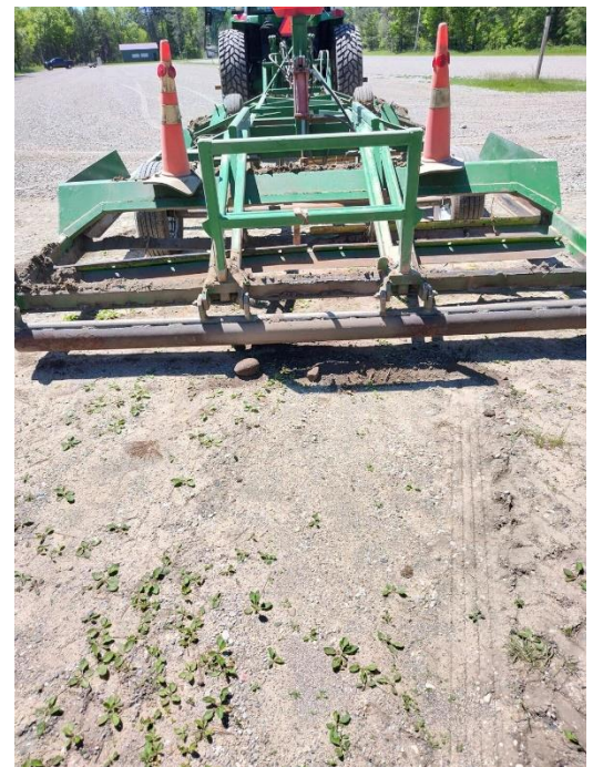
Russ and Greg spent an afternoon moving the drag from the 7610 to the 7410 so it is ready to grade WHEN we get the trail ok. Then Russ dragged the parking lot and a short piece of trail, trying out the new drag parts that John welded on Memorial Day. It looked good.
