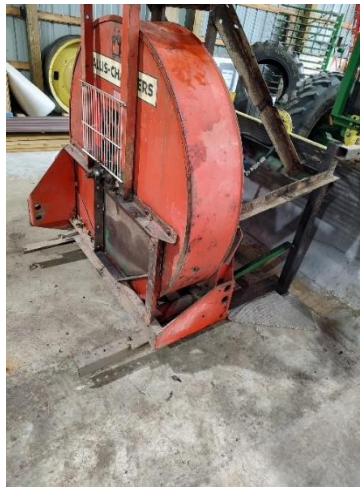
Our jury-rigged leaf blower was attached to the front of the 7410. It will blow leaves off the trail (esp EAST trail 6 that has tons of oak trees). Heavy leaf cover jams up the drags. Typically, one person drives a tractor to clear the trail and one follows to grade. Photo below shows how it clears the trail.
